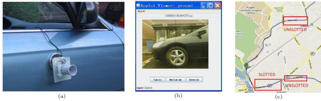
Figure 8: (a) An image of the ultrasonic sensor side-mounted on a car (b) the java applet used for recording ground truth from images. (c) The map of the data collection area (Mathur, et al., 2010)
