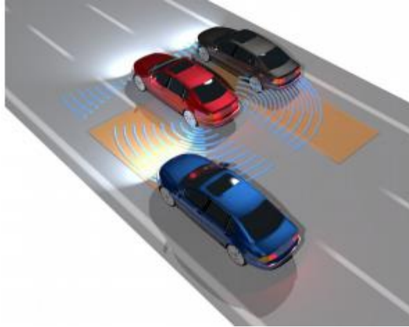
Figure 2: Installing several ultrasonic sensors on the latest cars. The arcs represent the ultrasonic sensors and their reach (Kohler, Connette, & Verl, 2013)
