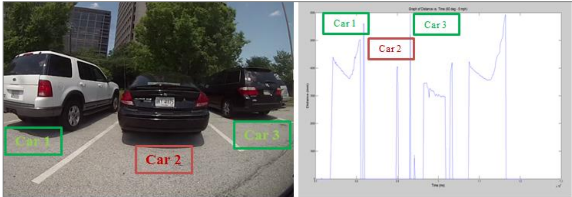
Figure 62: Example of black car that is not accurately detected by the sensor: (a) Ground truth from video and (b) sensor readings
